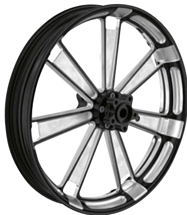
3 Machined front wheel 3.50 x 21" NEW
